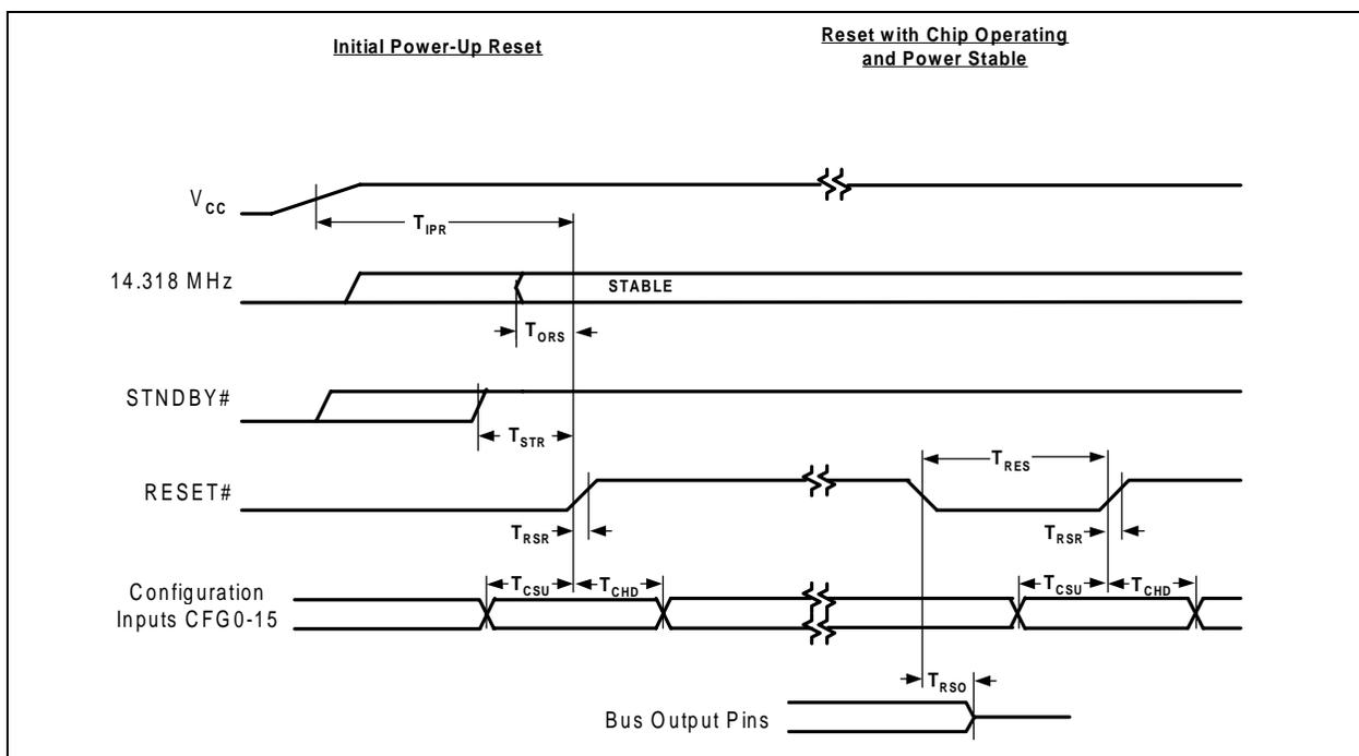
**Figure 3-3: Reset Timing**
