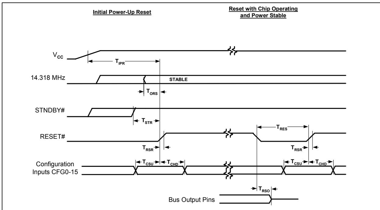
Figure 3-3: Reset Timing
