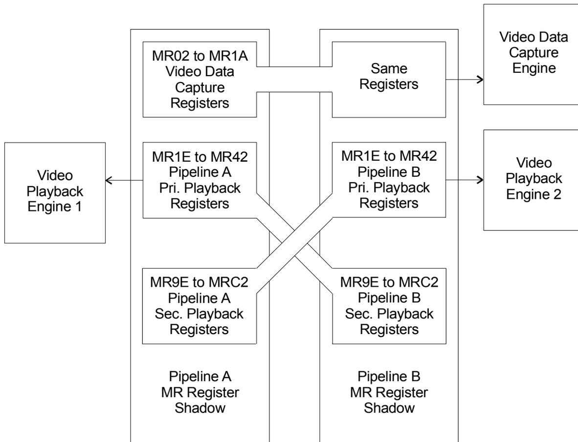
As shown, there is one set of registers for the video data capture engine, and this set is shared between both pipelines at register locations MR02-MR1A -- i.e., this one set of registers is accessible at register locations MR02-MR1A in both shadows of the MR register set.
