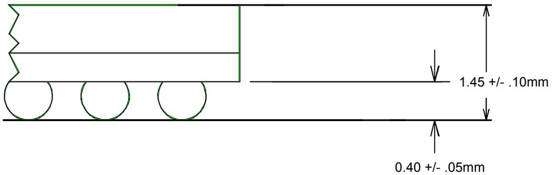
Figure 4-2: 256 Ball - Mini Ball Grid Array
