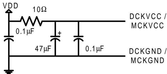
The suggested method for layout assumes a multi-layer board including VCC and GND planes. All ground connections should be made as close to the pin/component as possible. The CVCC trace should route from the graphics controller through the pads of the filter components. The trace should NOT be connected to the filter components by a stub. All components (particularly the nearest 0.1μF capacitor) should be placed as close as possible to the graphics controller.
