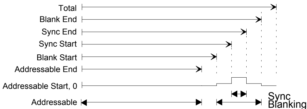
Figure 4-19. Display Timing Parameters
