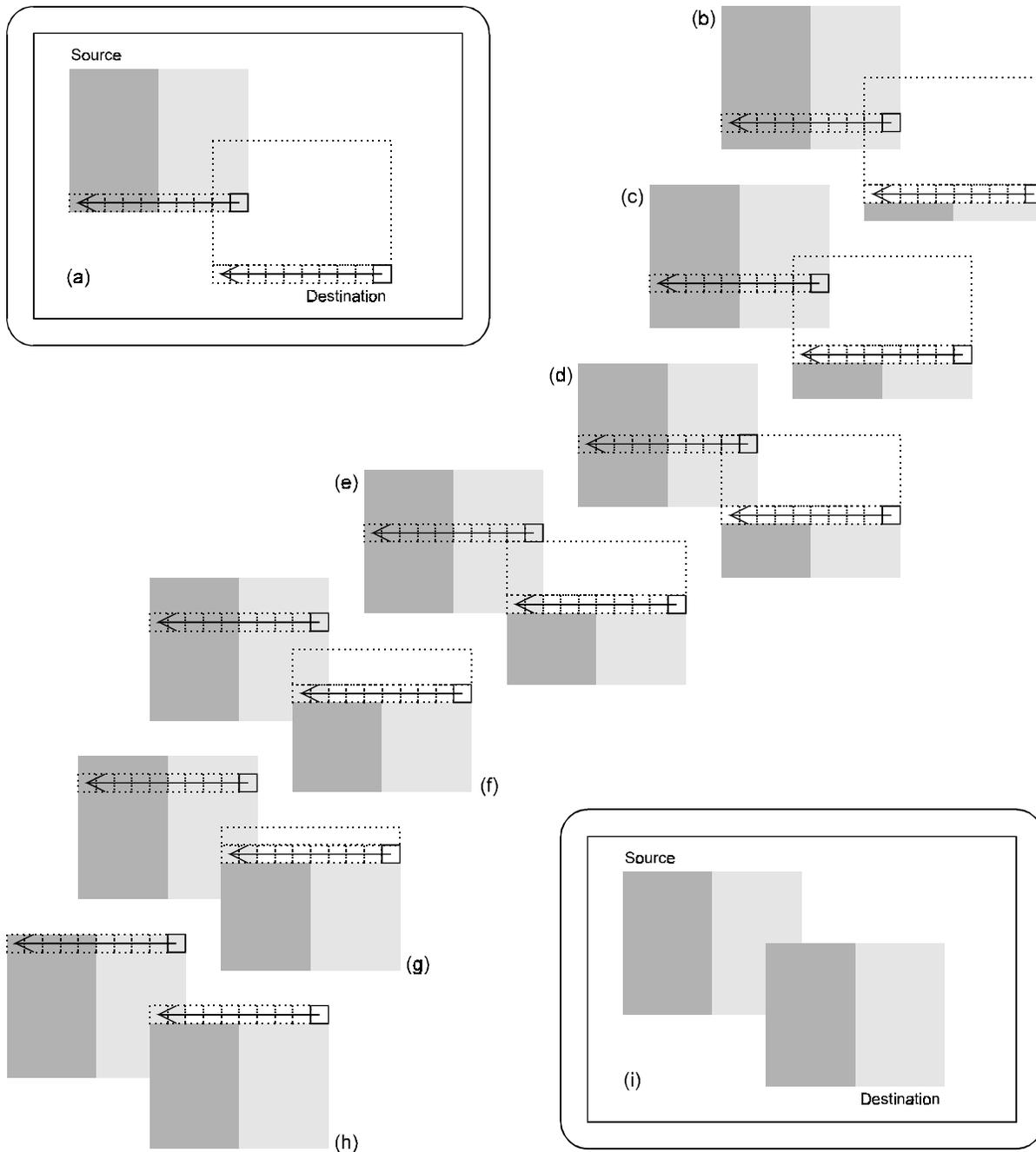
**Figure E-4: Correctly Performed BitBLT
